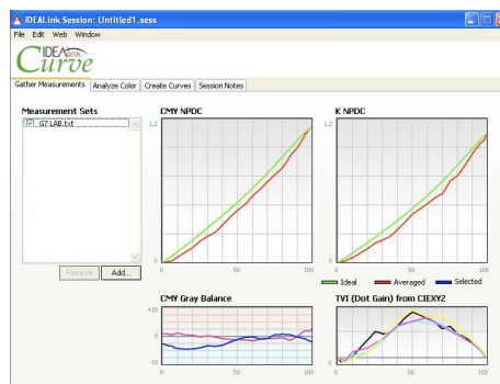
Figure2. Ideal (in green) and measured (in red) NPDC curves of cyan, magenta, yellow (left), and black (right)
