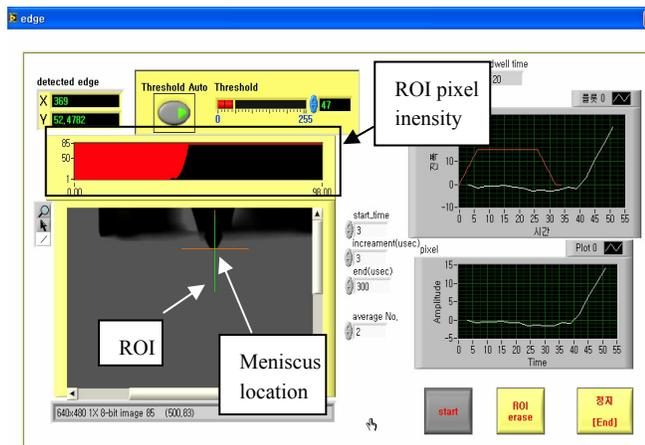
Figure 6. Meniscus location at a 50 μsec trigger delay.
