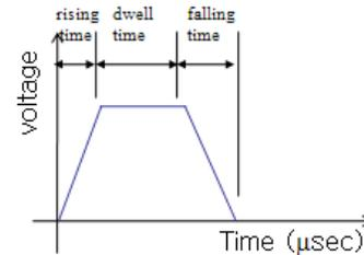
Figure 1. Typical waveform for the piezo inkjet.
