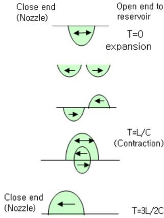
Figure 2. Pressure wave inside a print head.
