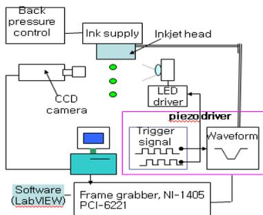
Figure 3. CCD camera system with a strobe LED.
