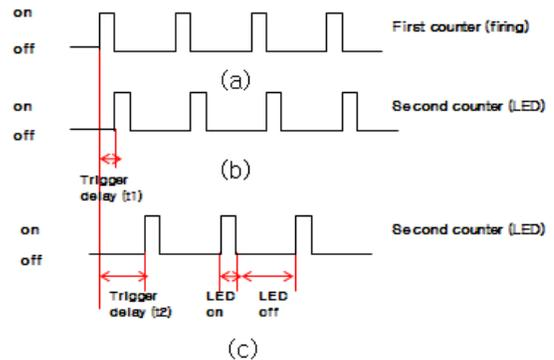
Figure 4 Time delay for the LED with respect to jetting signal.
