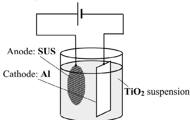
Figure 4. Schematic illustrations of the electrophoretic deposition
