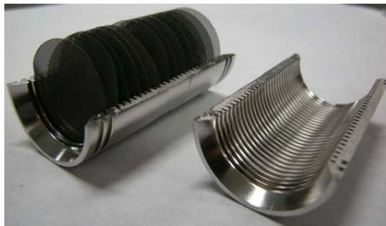
Figure 2. Cartridge system which includes SUS meshes
