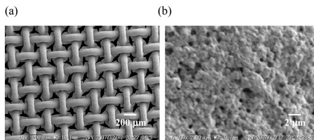
Figure 9. SEM pictures with different magnifications of electrophoretically deposited layers on SUS/Cr<sub>2</sub>O<sub>3</sub>
