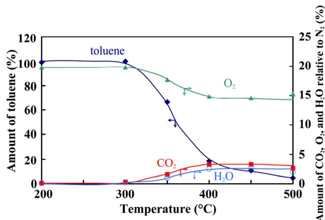
Figure 10. Decomposition of toluene in air with a cartridge system composed of ten meshes of SUS/Cr<sub>2</sub>O<sub>3</sub>/TiO<sub>2</sub> as a function of temperature
