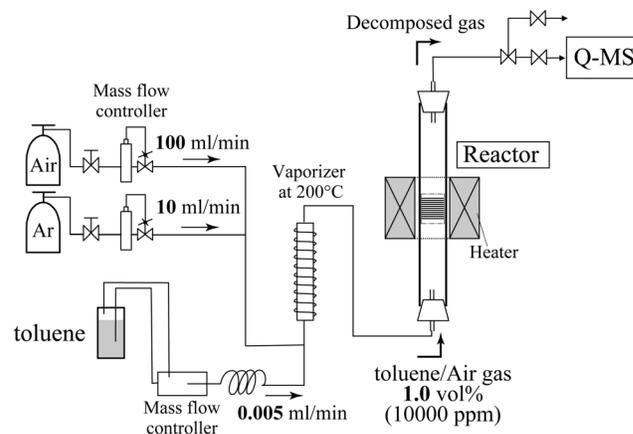
Figure 5. Schematic representation of the equipment for VOC decomposition
