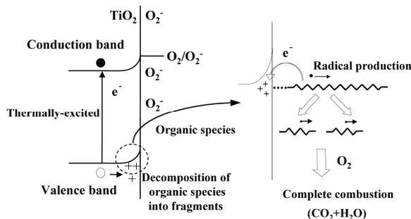
Figure 1. Decomposition process of PC at the “TiO<sub>2</sub>/PC” interface by means of thermally generated holes
