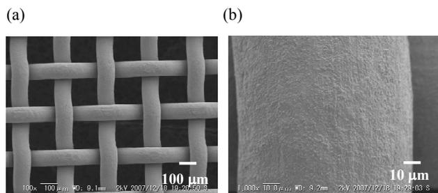
Figure 7. SEM pictures with different magnifications of the SUS/Cr<sub>2</sub>O<sub>3</sub> prepared by wet hydrogen
