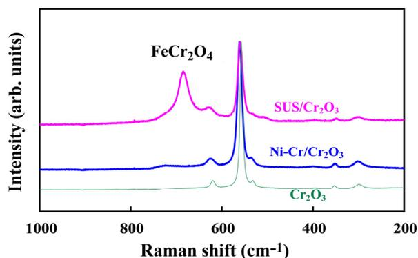
Figure 6. Raman spectra of SUS/Cr<sub>2</sub>O<sub>3</sub>, Ni-Cr/Cr<sub>2</sub>O<sub>3</sub>, and commercially available powdered Cr<sub>2</sub>O<sub>3</sub>
