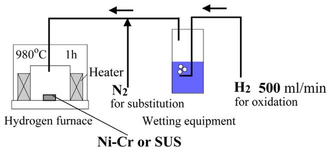
Figure 3. Equipment for oxidation of Ni-Cr wires or SUS meshes by wet hydrogen
