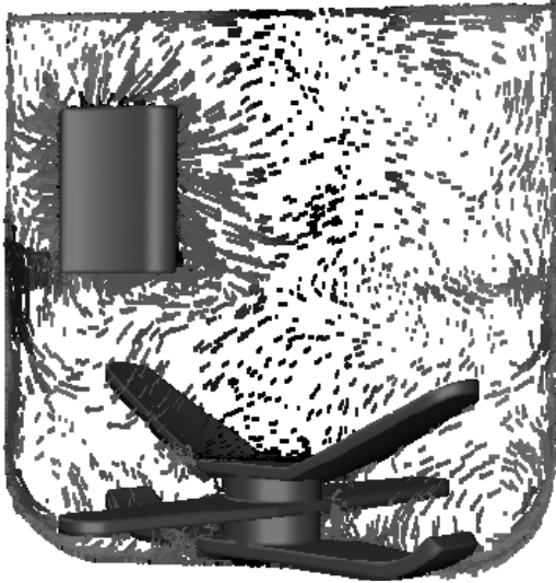
Figure 1. flow pattern in vertical plane (10L standard Henschel tool)
