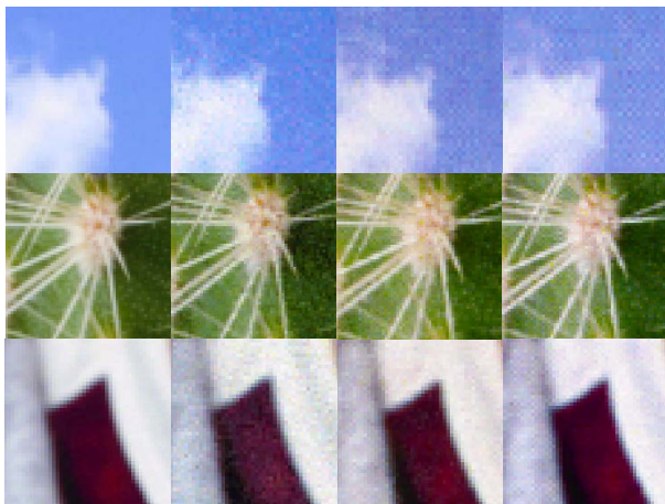
Figure 2. Five-time magnifications of typical digitized images. Papers from left to right: 26 (IJ), 20 (MP, printed with IJ), 20 (printed with EPG) and 8 (EPG).
