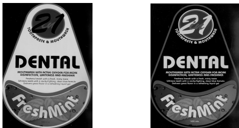
Figure 9. Clear substrate printed with CMYK + W ElectroInks.
