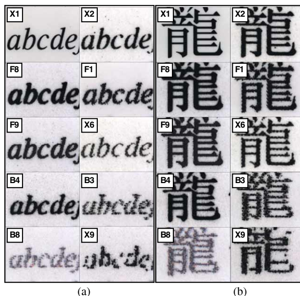
Figure 2. (a) 4 pt Times Roman fonts and (b) 9 pt Chinese characters. High-resolution images at 4680dpi. Note that the images in (a) and (b) are arranged in descending order of observer preference (left to right, top to bottom).
