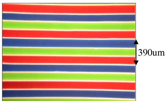
Figure 5. Optical microscopy photograph of a color filter fabricated by all ink-jet printing.
