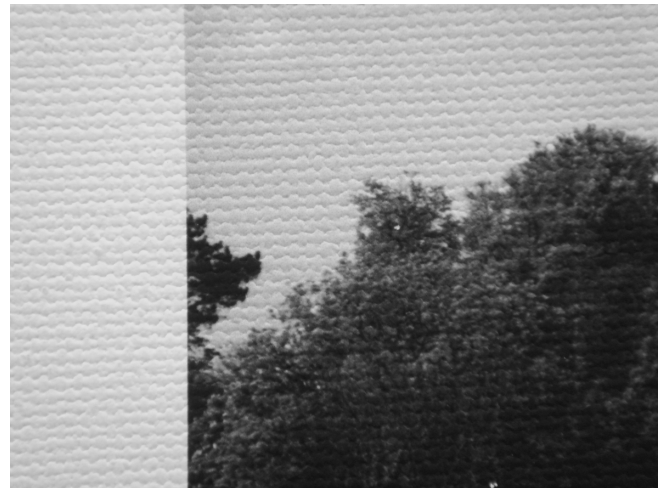
Figure 7: Exploded view of the HP cotton duck canvas both printed and unprinted surface, note the regular weave and even surface
