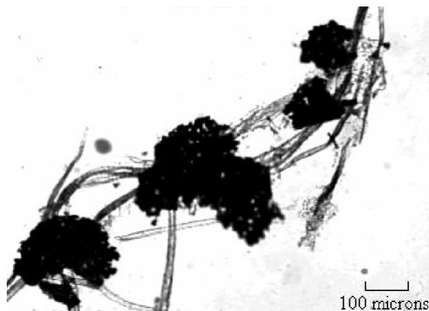
Figure 1 Toner particles attached to fibres after disintegration but prior to sonication.
