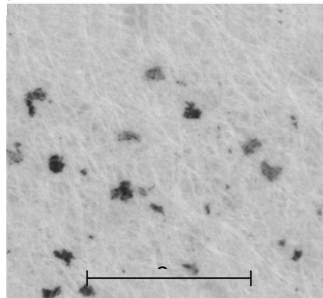
**Figure 5.** 75% half-tone dots, 10 minutes sonication, unwashed. The bar represents 2mm.
