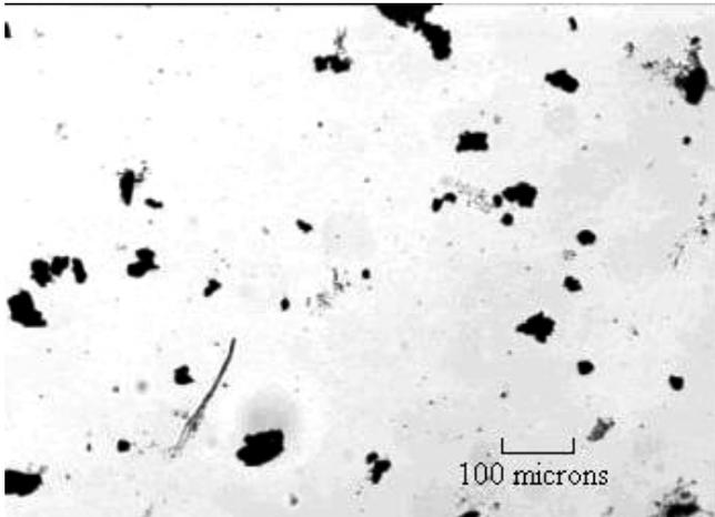
**Figure 2** Toner particles detached from fibres after 10 minutes sonication.
