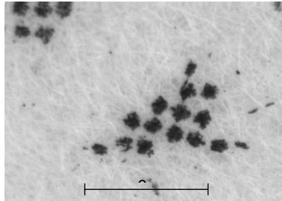
**Figure 4** 75% half-tone dots, unsonicated, unwashed. The bar represents 2mm
