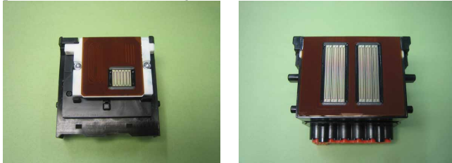
Figure 2. left) Printhead for PIXMA mini, four colors, 0.2inch print width right) Printhead for imagePROGRAF, 12 colors, 1 inch print width
