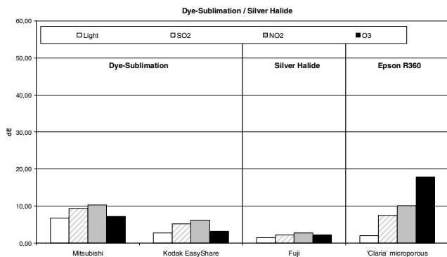
Figure 3. gas- and lightfading of pictures generated by dye-sublimation and the silver halide process vs. Epson R360
