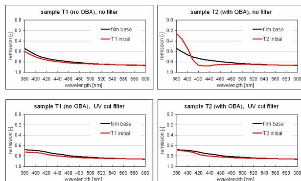
**Figure 1.** Spectral densitometer remission density (Spectrolino) for top left: sample T1 / no filter top right: sample T2 / no filter bottom left: sample T1 / UV cut filter bottom right: sample T2 / UV cut filter
