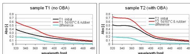
Figure 13. UV/VIS Absorbance Spectrum for sample T1 and T2
