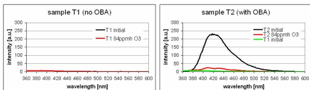
Figure 12. Fluorescence Emission Spectrum for sample T1 and T2
