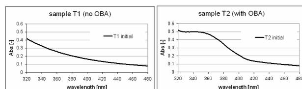
**Figure 2.** UV/VIS Absorbance Spectrum for sample T1, T2
