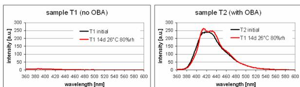
Figure 10. Fluorescence Emission Spectrum for sample T1 and T2
