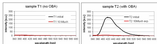
**Figure 5. Fluorescence Emission Spectrum for sample T1 and T2**
