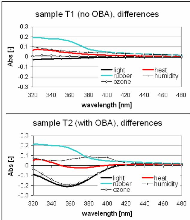
**Figure 15.** Difference UV/VIS Absorbance spectra for sample T1 and T2 where the spectra of the initial samples are subtracted from the spectra after the indicated treatments to show the induced spectral changes
