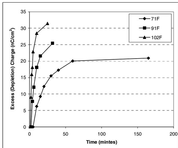
**Figure 4.** Excess charge as a function of dark rest time at 71, 91, and 102°F.
