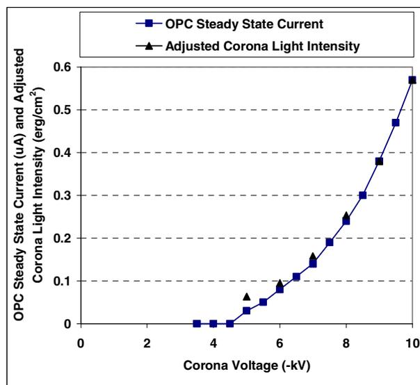
**Figure 5.** OPC steady-state current during charging, and the intensity of light emitted by the corona charger, as a function of corona voltage. The light intensity was determined by discharging the OPC with light from the corona using the known photosensitivity for a 775 nm exposure. The light intensity at -10 kV was normalized to the OPC current value at -10 kV.
