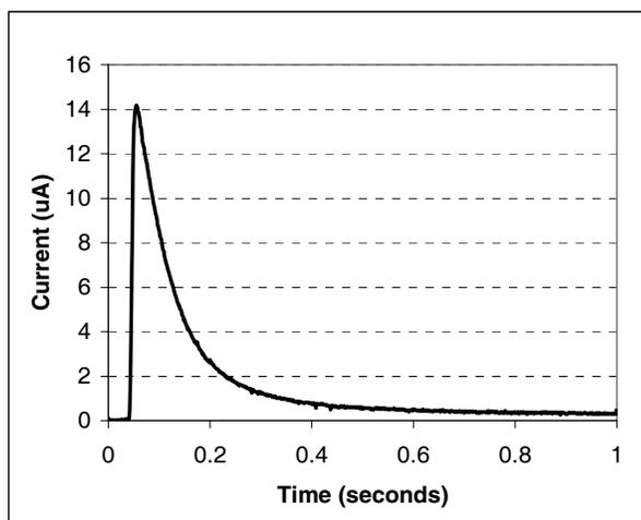
**Figure 1.** Charging current as a function of time for a 22  $\mu\text{m}$  bisphenol-A polycarbonate film with a grid potential ( $V_g$ ) of  $-500$  V.
