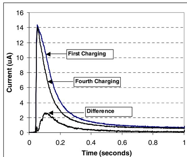
**Figure 2.** Charging current versus time for sequential charging of a near-infrared sensitive OPC. Prior to the first charging cycle, the film was exposed to laboratory lighting; after each charging cycle the film was dark rested for 8 min. The data shown is for the first and fourth charging cycle. Charging cycles 2, 3, and 4 were identical. Also shown is the difference between the first and fourth charging cycle.
