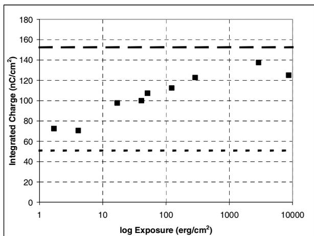
**Figure 3.** Integrated charging current as a function of 775 nm exposure ( $V_g = -700$ ). Exposure time (1, 10, 30 s) and light intensity (neutral density filters) were varied. The upper (dashed line) limit is the value obtained after exposure to laboratory lighting (gold fluorescent). The lower (dotted line) limit is the value obtained for the charge-depleted OPC.
