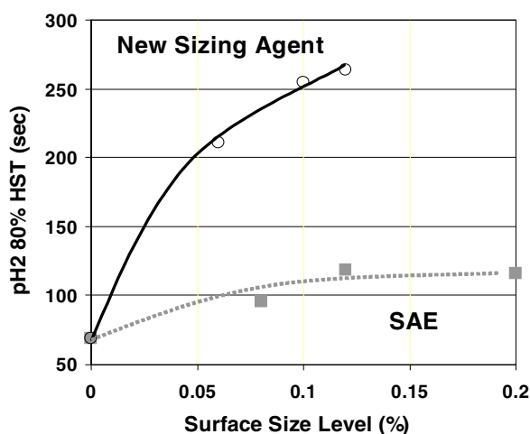
Figure 6. Surface Size Efficiency over Base Sheet with 0.046% ASA
