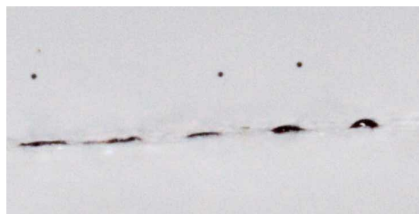
Figure 6. Inkjet ink droplets on copy paper during printing. The paper is moving from right to left at a paper feeding speed of 0.2 \text{ m s}^{-1} . An ink droplet is jetted every 1.2 ms. The rightmost droplet has just reached the paper as the picture was taken. Satellite droplets can be seen in the upper part of the picture.
