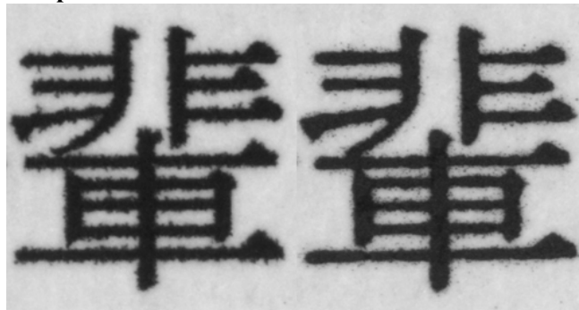
Figure 6. Plain paper Image of GelSprinter (High Quality mode) and Laser printer(MF7070)
