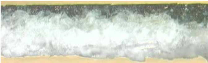
Figure 2. HP DeskJet 6122 black ink on everyday paper treated with color locking technology. Ink is retained on paper surface.
