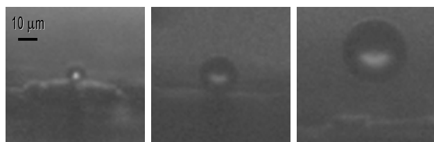
Figure 2. Satellite drop (left), primary planet drop (middle) and coalescent drop (right) of water.
