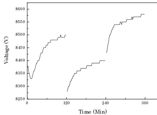
**Figure 4.** Dependence for voltage to maintain a constant discharge current (-0.5mA) over time for the temperature and relative humidity conditions listed in Table 1 for the negative discharge.
