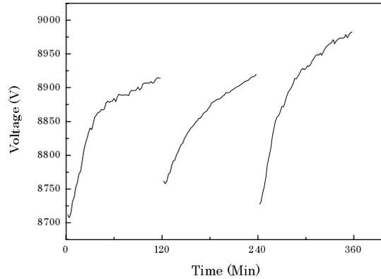
**Figure 10.** Dependence for voltage to maintain a constant discharge current (-0.5mA) over time for the relative humidity conditions listed in Table 2 for the negative discharge at 20 degrees.
