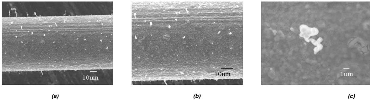
**Figure 11.** SEM micrographs of the wire anode for the relative humidity conditions listed to Table 1, (a)  $\times 750$ , (b)  $\times 1500$ , (c)  $\times 7500$ . The discharge time was 360minutes.
