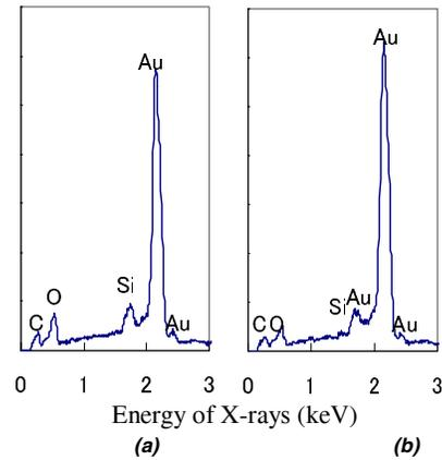
**Figure 7.** Results of qualitative analysis by EDS for temperature and relative humidity conditions listed to Table 1, (a) in positive corona discharge case, (b) in negative corona discharge case.
