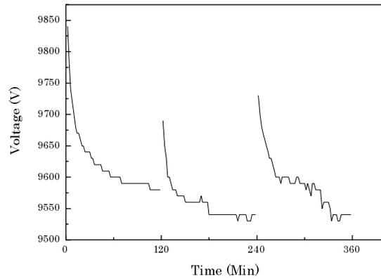
**Figure 3.** Dependence for voltage to maintain a constant discharge current (+0.5mA) over time for the temperature and relative humidity conditions listed in Table 1 for the positive discharge.
