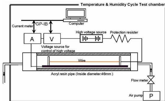
Figure 1. Schematic diagram of the experimental system.
