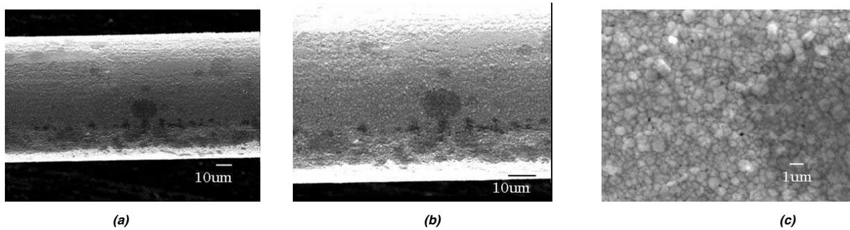
**Figure 12.** SEM micrographs of the wire cathode for the relative humidity conditions listed to Table 2, (a)  $\times 750$ , (b)  $\times 1500$ , (c)  $\times 7500$ . The discharge time was 360minutes.
