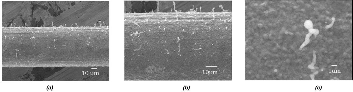
**Figure 5.** SEM micrographs of the wire anode for temperature and relative humidity conditions listed to Table 1, (a)  $\times 750$ , (b)  $\times 1500$ , (c)  $\times 7500$ . The discharge time was 360 minutes.
