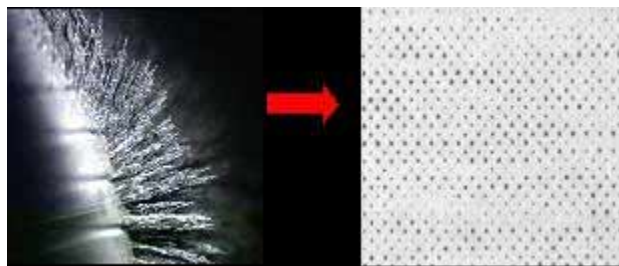
Figure 1 Illustration of magnetic brush structure and high frequency noise in a halftoned image.
