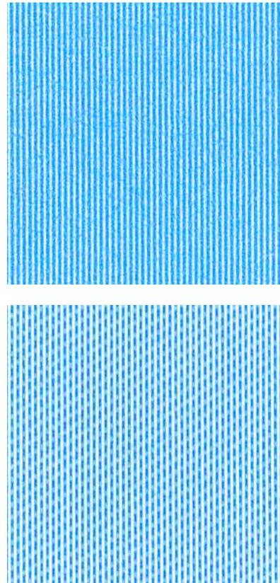
**Figure 4. Sample cyan color line feature. Deskjet 5440 (top) and Laserjet 4700dn (bottom) are shown..**
