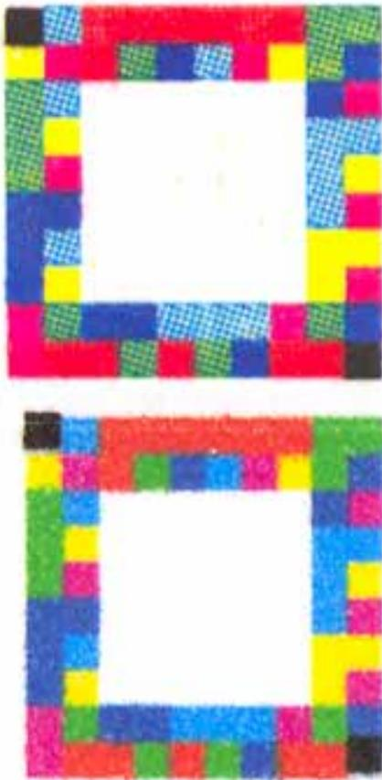
Figure 6. Laserjet, size 16 pixels (above); TIJ, size 16 pixels (below).
