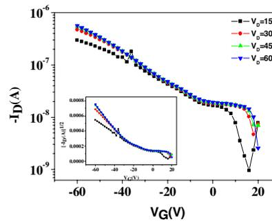
Figure7. Characteristics of a ring-ridge patterned organic thin film transistor with pentacene as the active layer
