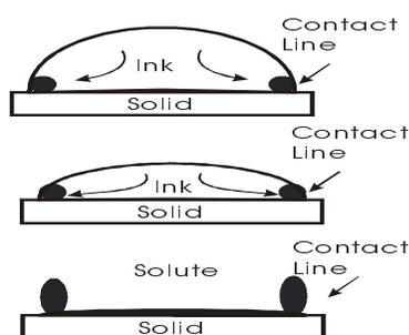
Figure 1. Ring-shaped forming mechanism(□)
