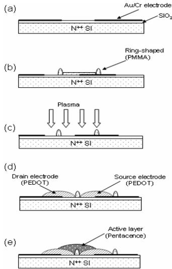
Figure4. Schematic illustration of the process flow of ring ridge patterned organic thin film transistors
