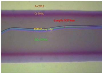
Figure5. The microscopy of a coffee ring after plasma etching
