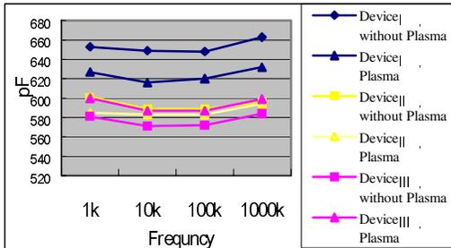
Figure6. The resulting capacitance of doped Si/SiO<sub>2</sub>/Al devices with and without plasma treatment on the oxide layer
