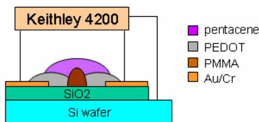
Figure 3. The structure of the organic thin-film transistor device (OTFT) with a ridge of PMMA ring edge
