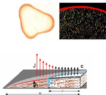
Figure 2. Coffee Ring forming mechanism(□)
