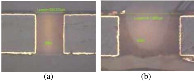
Fig3. Vertical cross section of (a) 200µm diameter and (b) 420µm vias on 250µm thick substrate which is processed using process of Fig.2.
