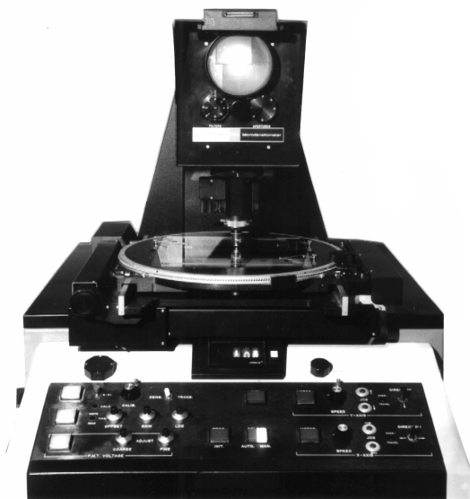
Figure 3 A Perkin Elmer PDS 1010A microdensitometer
