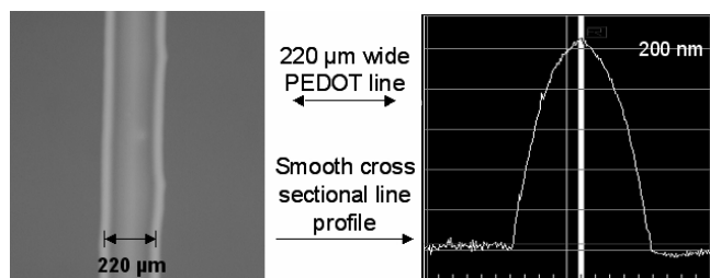
Figure 4. Optical image and line profile of an electrode line inkjet printed with a modified Baytron P Jet HC dispersion
