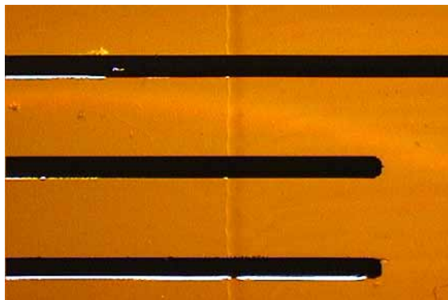
Figure 6: Wet out of Cabot 50 wt% Prototype Silver Ink on DuPont™ Kapton® (left portion of image) and on Inkjet Printed and Cured Chisso PI PIN-6100-001 Ink Sample (right portion of image)
