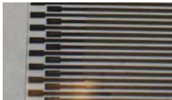
Figure 1: Inkjet Printed Nickel Electrodes and Interconnects (down to 100 micron line width)
