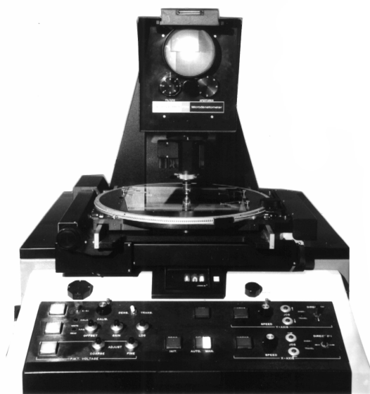
Figure 1 A Perkin Elmer PDS 1010A microdensitometer
