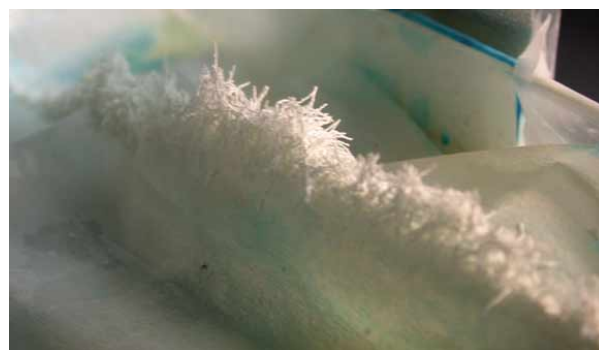
Fig.2 High thixotropic ink discharged down and its accumulation behavior presented.
