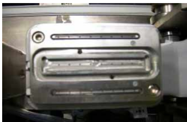
Fig.4 Top view of maintain mechanism, two suction areas were at the top of picture, and a flushing area located at the center area, the bottom area was a capping area.
