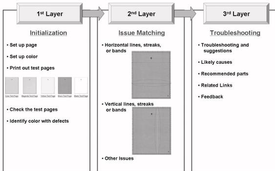
Figure 7. The PQTS three-layer architecture model.
