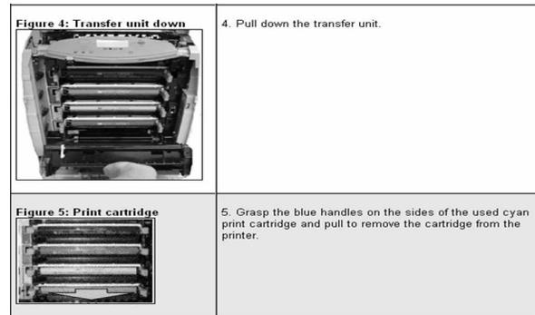
Figure 8. Segment of the replacing cartridge procedure.
