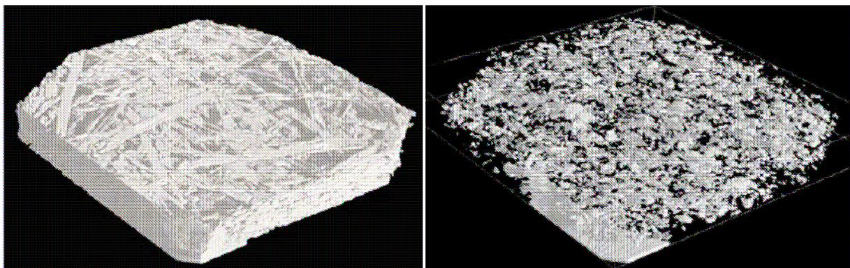
Fig. 10: 3D view of the fibrous structure and fillers localisation within the structure.
