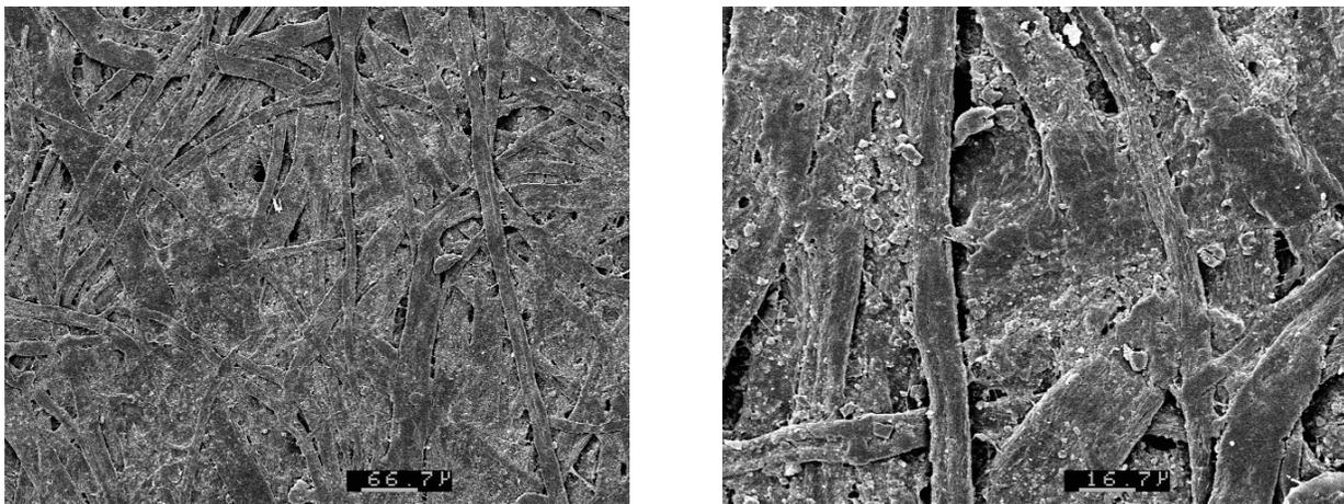
Fig. 2: Scanning electron microscopy: paper 2 (scale: 66.7 and 16.7 microns, respectively)
