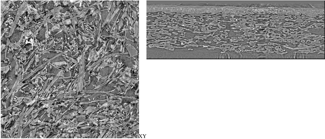
Fig. 8: Paper 3 (in plane (981  $\mu\text{m}$  \* 981  $\mu\text{m}$ ) and (292  $\mu\text{m}$  \* 95.9  $\mu\text{m}$ ) cross views)
