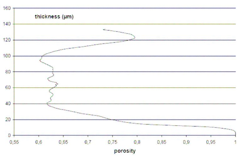
Fig. 9: Porosity profile (thickness direction) for paper 1
