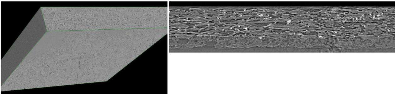
Fig. 6: Paper 1 (3D (981  $\mu\text{m}$  \* 981  $\mu\text{m}$ ) and cross section (371  $\mu\text{m}$  \* 70  $\mu\text{m}$ ) views)
