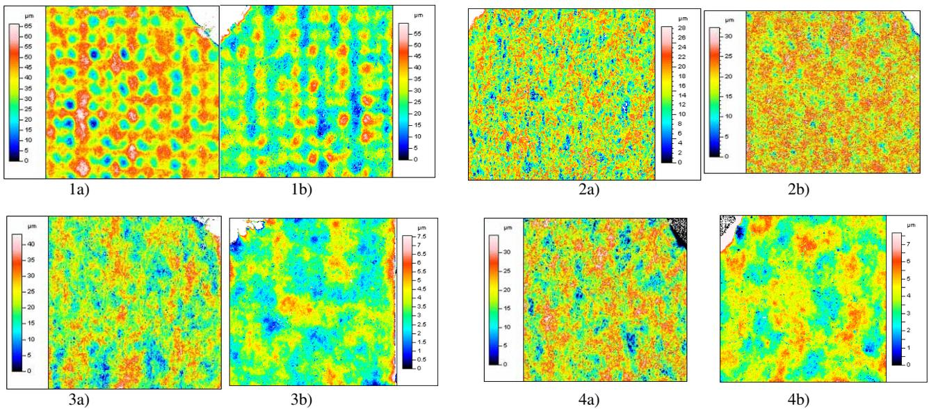
Fig. 3: Optical profilometry: two sidedness effect (Paper 1 to 4, resp. side a and b) – Measurements on 6x6 mm<sup>2</sup>
