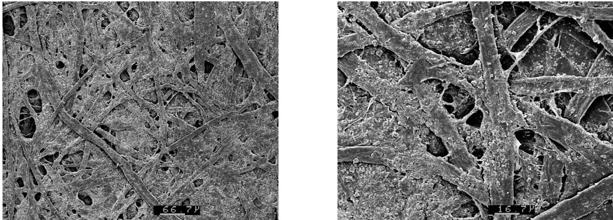
Fig. 1: Scanning electron microscopy: Paper 1 (scale: 66.7 and 16.7 microns, respectively)
