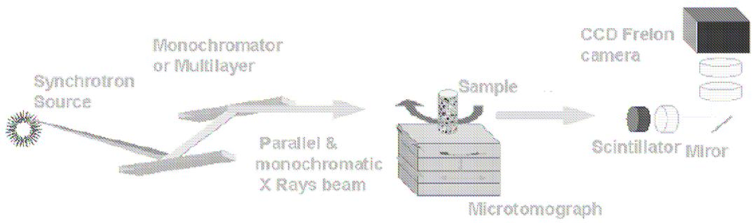
Fig. 4: Schematic view of the data acquisition involved at the ESRF installation
