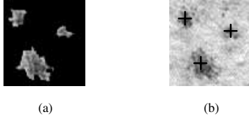
Figure 4. (a) binary mask image and (b) dot centroids
