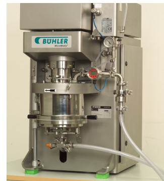
Fig. 6: Nano-grinding in pilot-size mill MicroMedia ® P1 (from ceramics)
