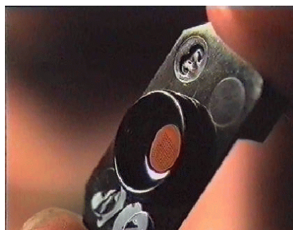
Figure 21. Disposable diagnostic test that contains up to 100 tests printed using ink-jet technology.
