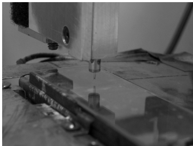
Figure 2. Inkjet print head positioned over a glass substrate.
