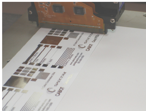
Figure 3. Inkjet printing of Cabot Inkjet Printable Silver Conductor on paper using Spectra-SE128 printhead.
