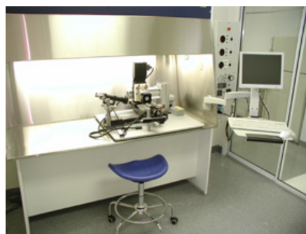
Figure 2. Desktop JetLab® system attached to a tissue culture hood for sterile manufacturing.
