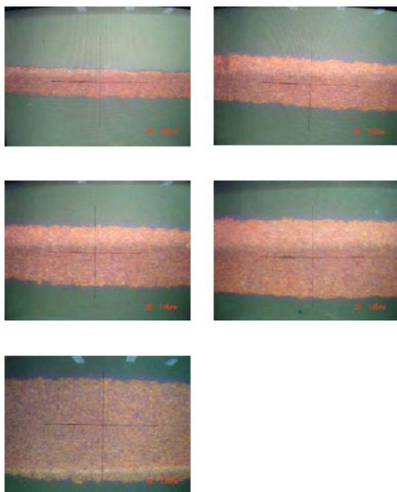
Figure 6 pictures of different wire width ( $75\mu\text{m}$ ,  $115\mu\text{m}$ ,  $150\mu\text{m}$ ,  $185\mu\text{m}$ ,  $225\mu\text{m}$ )
