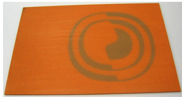
Figure 4. A graphite sheet with copper and iron powder (dark) deposited on it.
