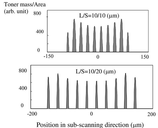
Figure 8. Line/Space-dependence toner deposition of multi-line of  $L/S = 10/10, 10/20$  micrometers.
