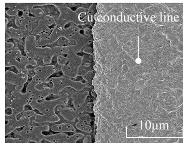
Figure 4. The SEM image of edge of Cu conductive line.
