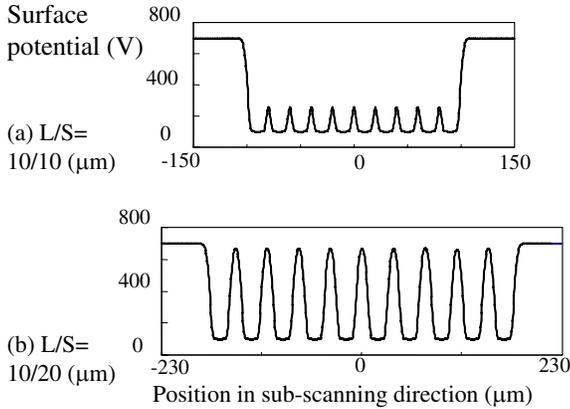
Figure 6. Potential distribution of multi-line of  $L/S = 10/10, 10/20$  micrometers, respectively ( $V_0 = 700$  V).
