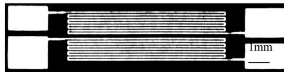
Figure 5. Wiring patterns for measuring the resistance.
