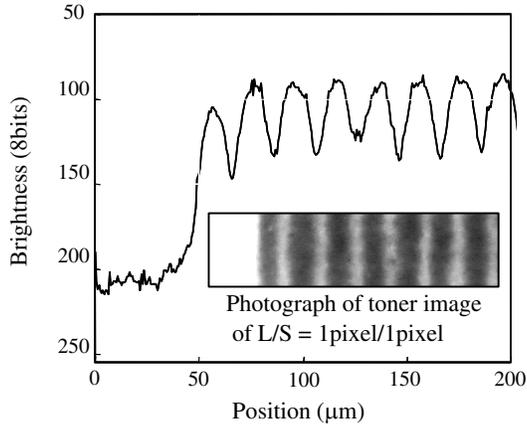
Figure 9. Experimental result using 2540 dpi LSU; brightness for each line of the  $L/S = 1\text{pixel}/1\text{pixel}$  multi-line formed on the paper.
