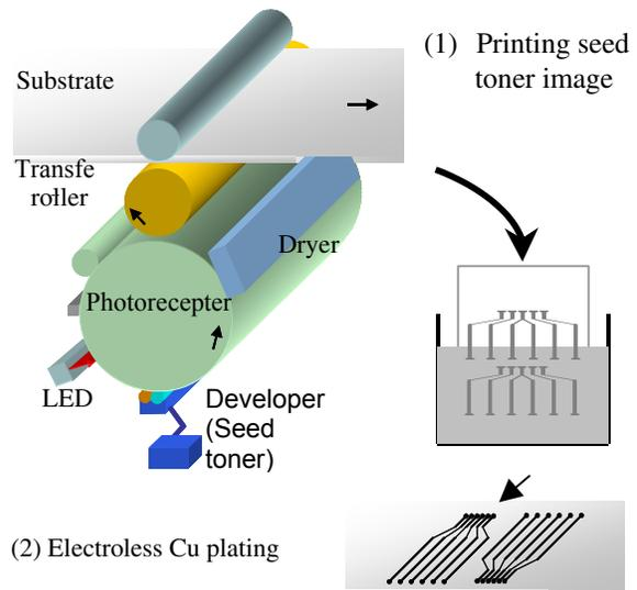
Figure 1. New process of fine pitch pattern formation using liquid toner electrophotography technology.
