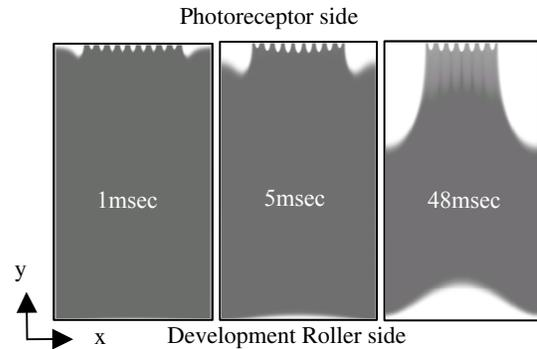
Figure 7. Time-dependence toner distribution of multi-line of  $L/S = 10/10$  micrometers in development gap ( $V_b = 400$  V).
