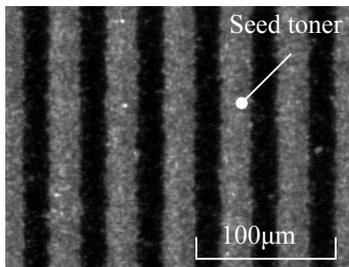
Figure 2. Fine pitch pattern of L/S = 1pixel/1pixel using seed toner printed by liquid toner electrophotography.
