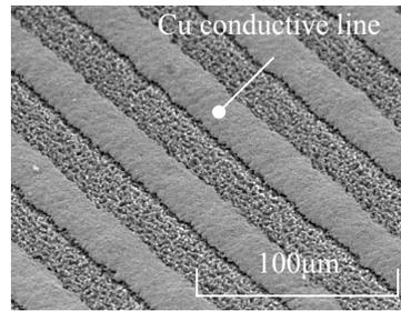
Figure 3. The SEM image of Cu conductive pattern of 4 micrometers thickness deposited by electroless plating.
