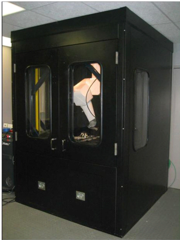
Figure 6. Photograph of a 3D conformal direct write fabrication cell.
