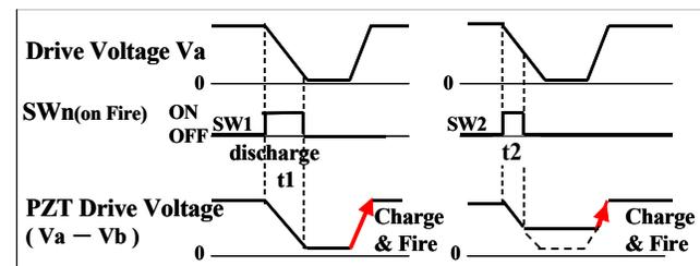
Figure 5. Nozzle Trimming Principle
