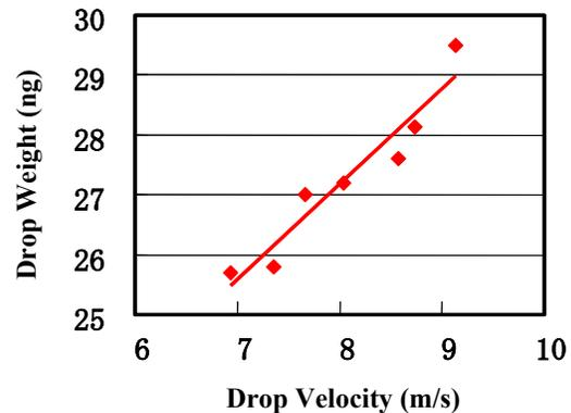
Figure 8. Drop Weight vs. Drop Velocity for non-average nozzles
