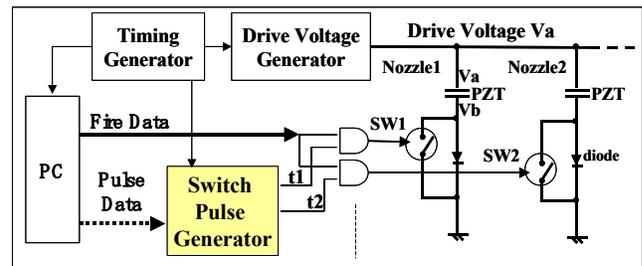
Figure 4. Structure of New Drive Electronics
