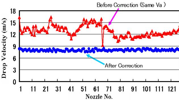
Figure 9. Drop velocity vs. nozzle number before & after velocity correction by trimming.
