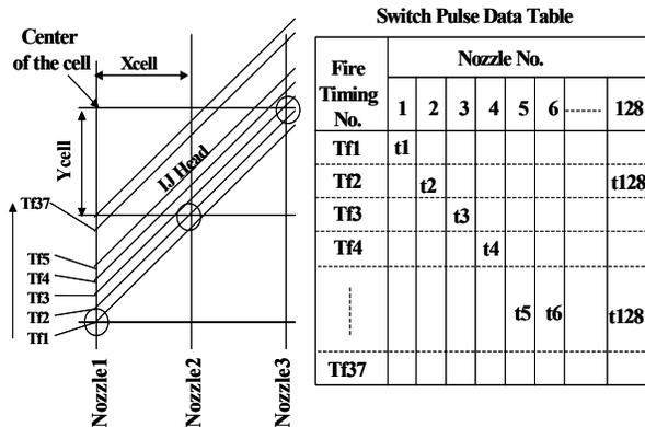
Figure 6. Fire Timing & Switch Pulse Data Table
