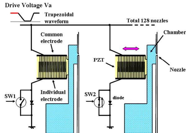
Figure3. Inkjet Structure and Principle
