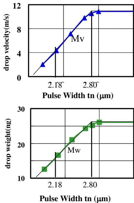
Figure 7. Drop Velocity & Weight vs. Switch Pulse Width  $T_n$  For Average Nozzles
