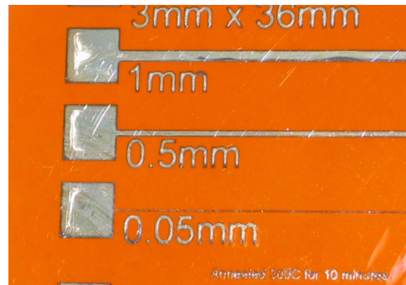
Figure 10. Ink jet printed silver conductive ink on a polyimide substrate (Sample courtesy of Cabot Corp.).
