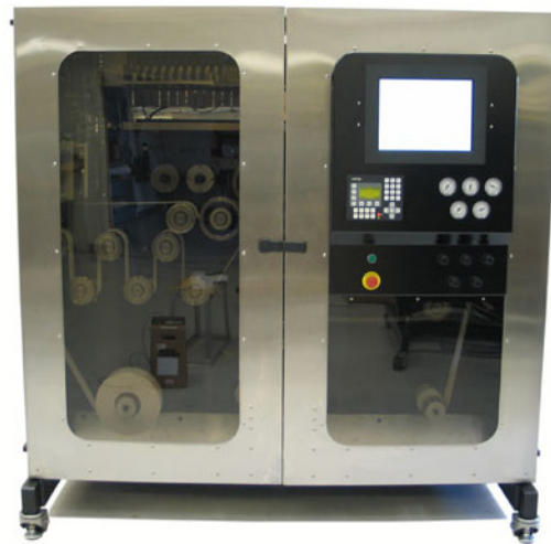
Figure 7. Digital Web Press with eight Xaar print heads.
