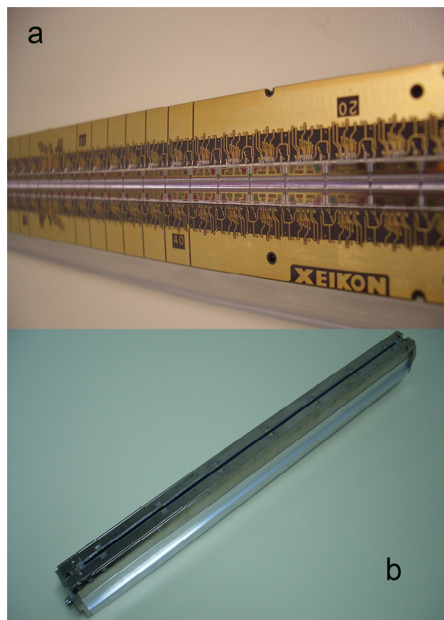
Figure 4. Photographs of prototype 520 mm array a) without lens system b) with Selfoc lens mounted
