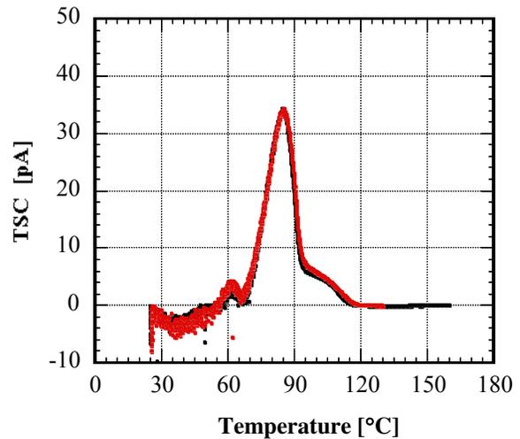
Figure 7. TSC spectrum for toner R corona charged (-5kV).
