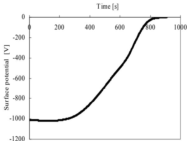
Figure 11. TSCD curve for acrylic powder corona charged (-1kV)
