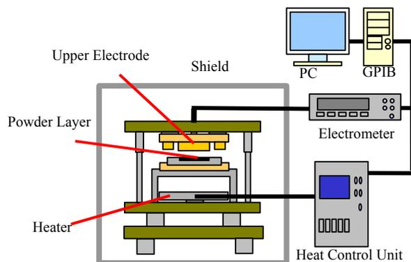
Figure 1. Experimental setup for TSC measurements.
