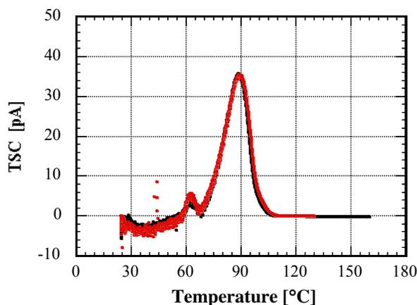
Figure 10. TSC spectrum for toner R+CB+CCA corona charged (-5kV).
