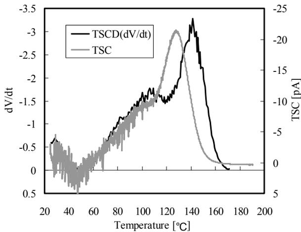
Figure 14. TSCD spectrum for acrylic powder corona charged (1kV).
