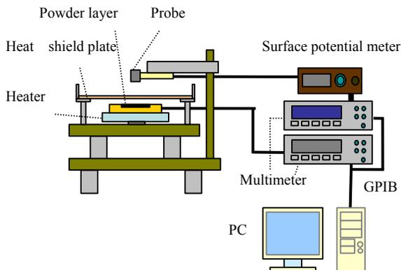
Figure 2. Experimental setup for TSCD measurements.
