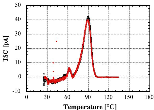
Figure 9. TSC spectrum for toner R+CCA corona charged(-5kV).
