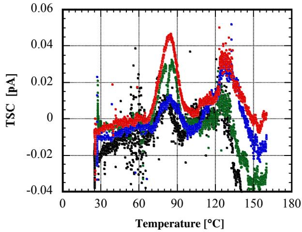
Figure 3. TSC spectrum for toner R tribocharged.
