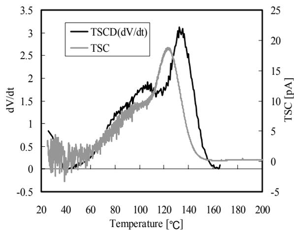
Figure 15. TSCD spectrum for acrylic powder corona charged (-1kV).
