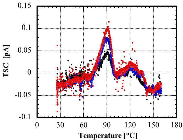
Figure 4. TSC spectrum for toner R+CB tribocharged.
