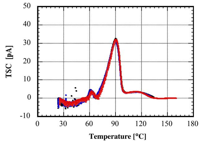
Figure 8. TSC spectrum for toner R+CB corona charged (-5kV).
