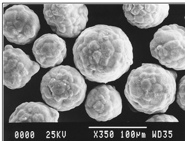
Figure 1. SEM photograph of carrier for P-type carrier
