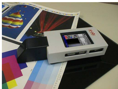
Figure 6. DIAS – Distinctness of Image Analysis System
