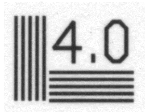
Figure 4b. Resolution target 4.0 scanned at 1600dpi
