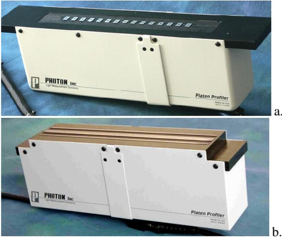
Figure 2. Platen Profiler developed by Photon: a) Discrete design for Laser Printheads; b) "Continuous" design for LED Printheads
