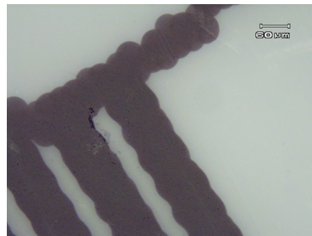
Figure 10. Coating thickness 34 \mu\text{m} (0.1 \mu\text{m} line block printing 200 times optical microscope)
